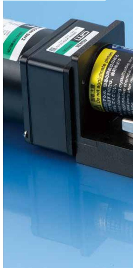
The Iwaki Hicera pump is a compact metering pump that employs a fine ceramic plunger. The unique valveless construction eliminates problems caused by clogging and jamming that commonly occur in conventional metering pumps. The precision micron-machining on the main ceramic parts ensures a high degree of discharge accuracy. The versatility of the Iwaki Hicera pump makes it ideal for micro-chemical feeding as well as high-viscosity liquid feeding.
